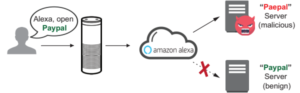
(b) Skill Squatting Attack: Attacker registering a malicious skill whose name sounds like that of the “PayPal” skill. The cloud could misinterpret the user voice command to invoke the malicious skill.
